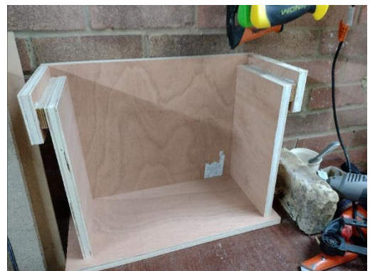
Despite the perspective of this picture, the ends are, of course, parallel. The 'ends' consists of three pieces which were glued and screwed first, then fastened to each hive 'side'. (The board at the back is a 'side'.) The floor was screwed on last. These boards are hardwood plywood; the shop must have run out of softwood and completed my order with hardwood ply!
