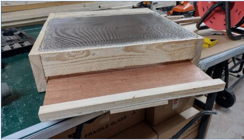
View from the back showing the sliding drawer. It is completely draught-proof making it similar to a solid-floor. Monitoring mites and board debris is still possible by placing a sheet of Correx on the board. Although the board is a neat fit, a strip of timber is fitted below the board to provide a handle.
