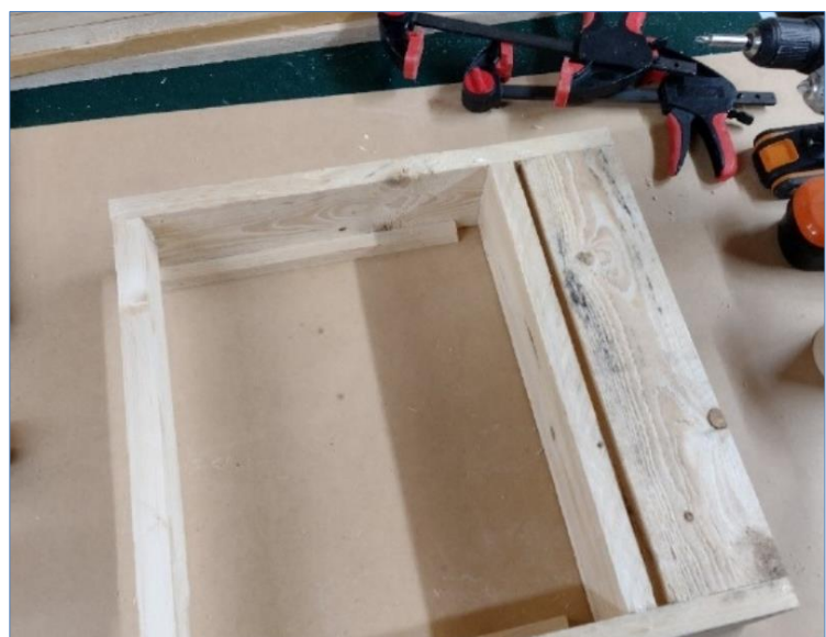
View from above before the mesh is stapled on. The bees enter the hive from underneath through the 8mm slot near the right edge.
