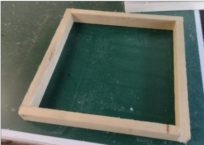
Above, an eke / frame from 50x25mm timber using four pieces each 435mm long, screwed and glued together.
